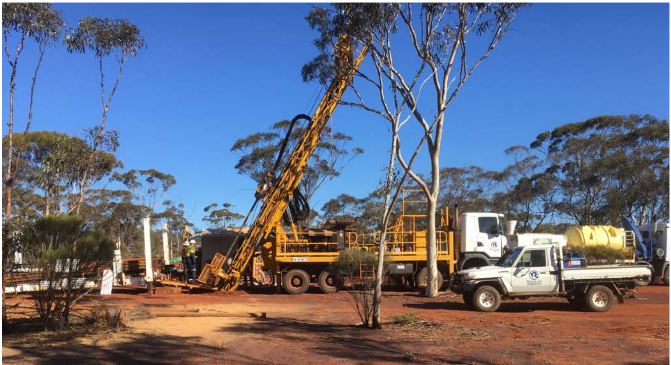
Figure 1: Drilling the first diamond holes into Myhree during the September 2019 quarter.
