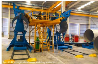
Two K-TIG longitudinal seam welding stations.
