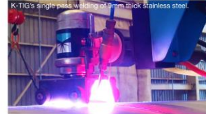
K-TIG's single pass welding of 9mm thick stainless steel.
