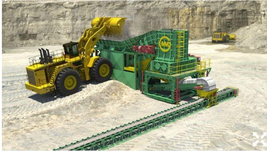
Figure 24: Mining process – silica sand loaded and screened
