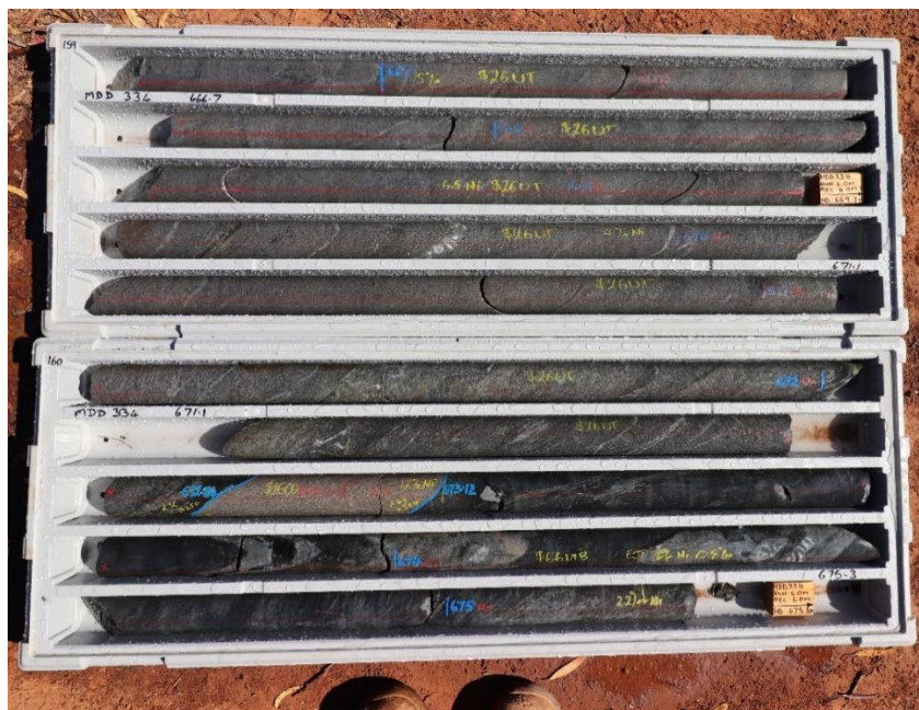
Figure 1: MDD334 core photo showing massive and heavy matrix nickel sulphides
