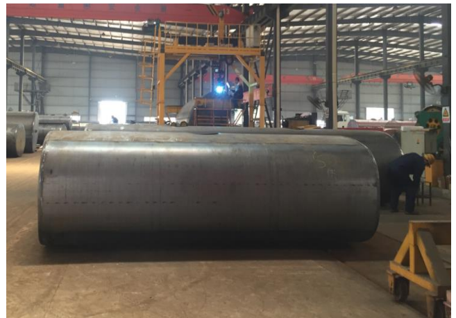
Water Truck tank being fabricated
