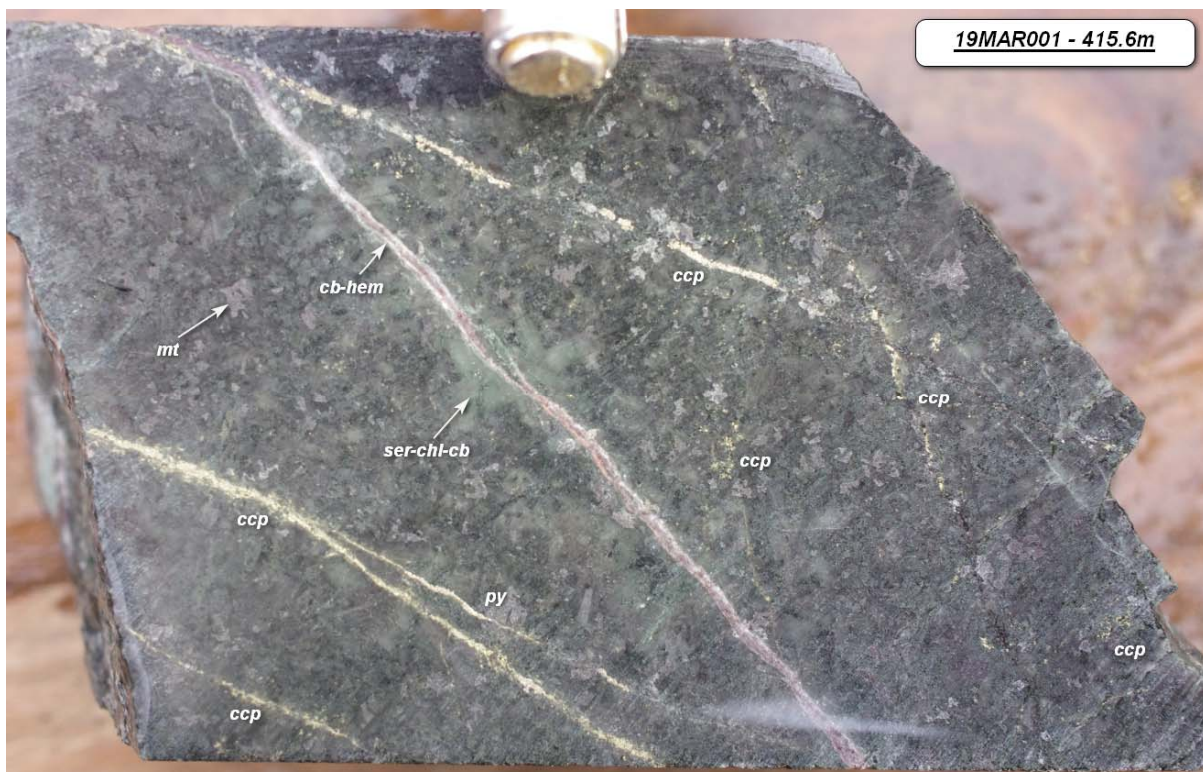
Figure 10 19MAR001 at 415.6m depth. Chalcopyrite and pyrite vein networks overprinting sericite-chlorite-carbonate-magnetite altered diorite.
