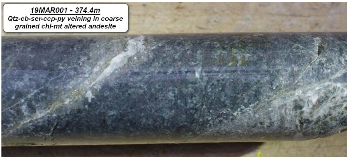
Figure 8 19MAR001 at 374.4m depth. Quartz-carbonate-sericite-chalcopyrite-pyrite veins in coarse grained chlorite-magnetite altered diorite.
