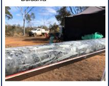
Buldania drill core showing coarse spodumene crystals
