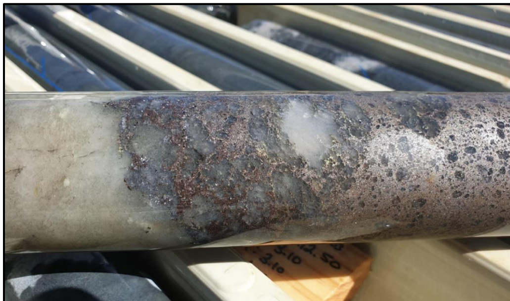
Figure 3. SPWDD003 221.1m to 221.3 Close up of contact between quartz vein and sulphidic breccia
