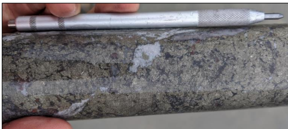
Photo 1. Massive pyrite with minor chalcopyrite vein at 860.5m in SMD045W2.
