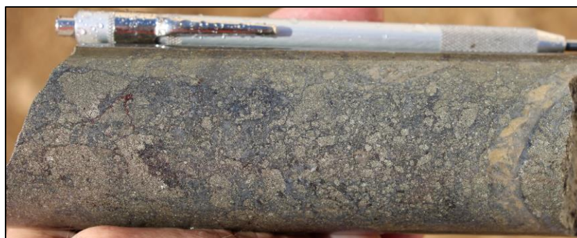
Photo 2. Pyrite breccia with quartz bornite and chalcocite infill at 1,133m in SMD045W2.
