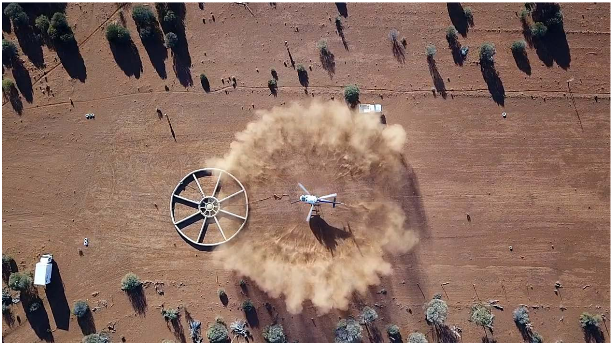
NRG Helicopter - Time domain EM survey data capture Bottle Creek 2019
