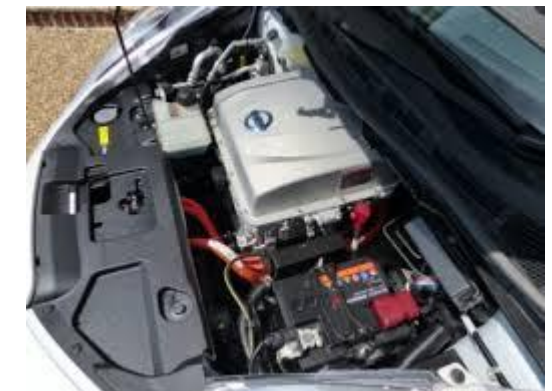
Under the bonnet of a Nissan Leaf – note the lead-acid battery centre bottom (image: autonews.uk.com)
