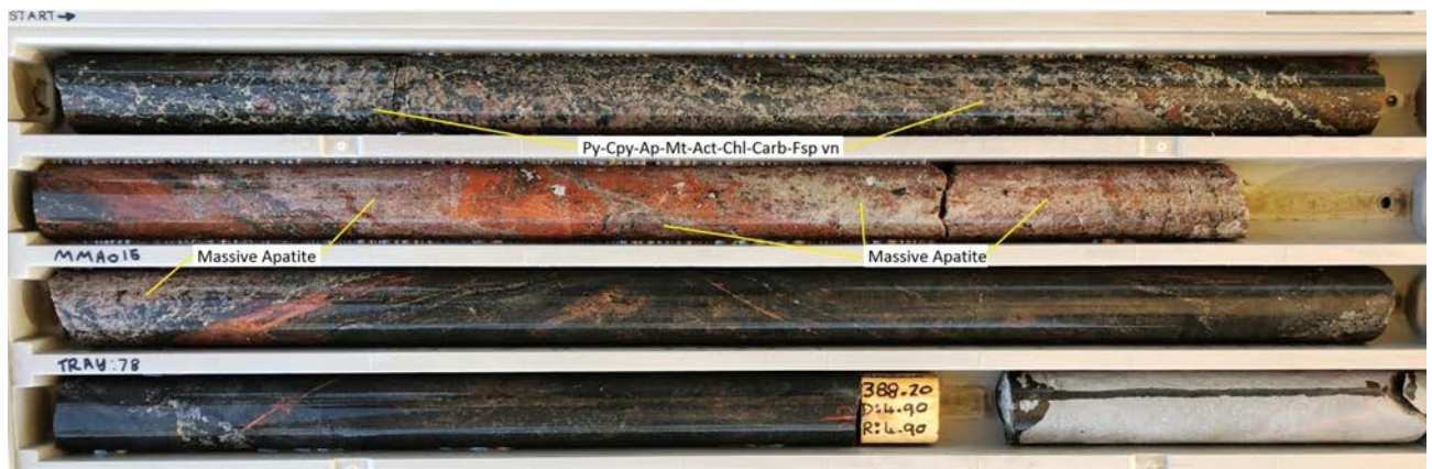
Figure: Drill hole MMA015. Massive pyrite-chalcopyrite-magnetite-actinolite-chlorite-carbonate-apatite vein (385.2-387mDH) returned 2m @ 0.39 % Cu from 385 m downhole.
