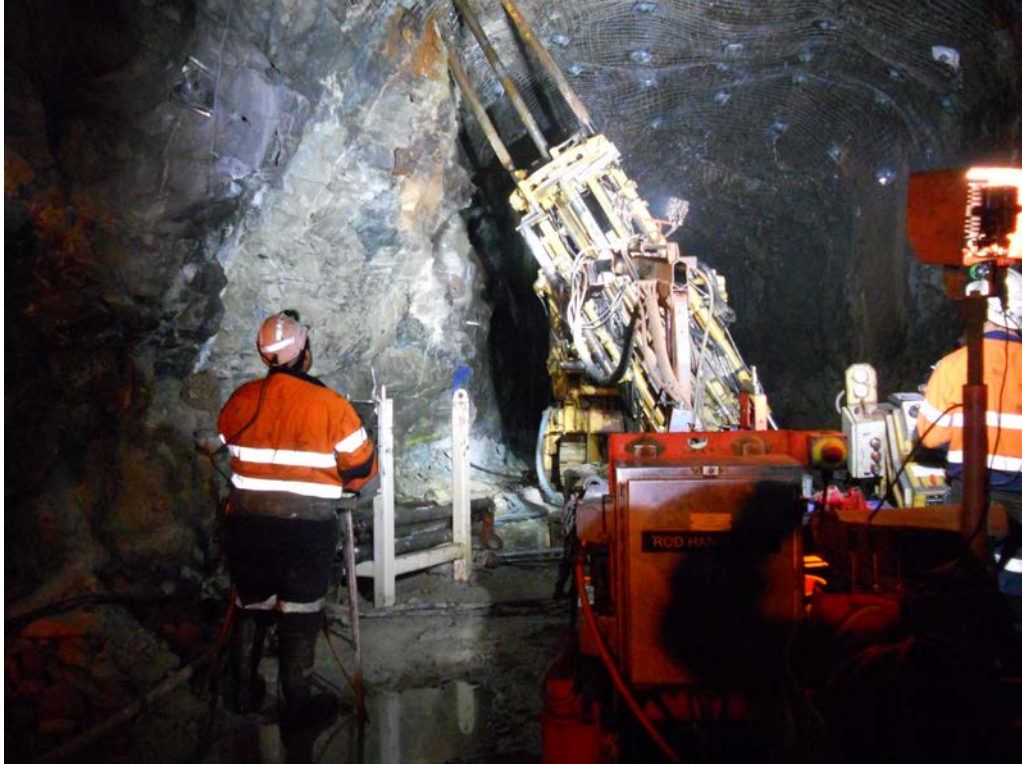
Figure 3- Underground RC drill rig in use
