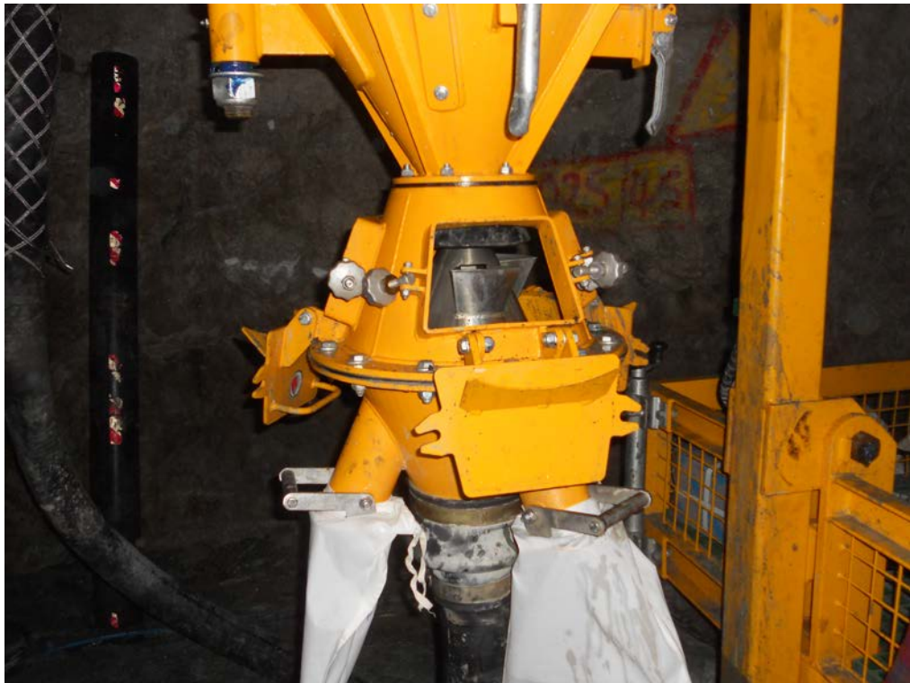
Figure 4- Purpose built underground RC rotary splitter
