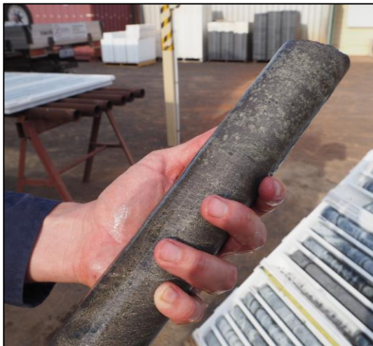
Photo 1 – 3: Massive pyrrhotite – pentlandite (nickel sulphide) – pyrite – chalcopyrite over 1.77m in drill-hole SNDD005 at Saint Patricks: 1.77m @ 6.72% Ni, 0.27% Cu and 0.13% Co from 227.31m down-hole.
