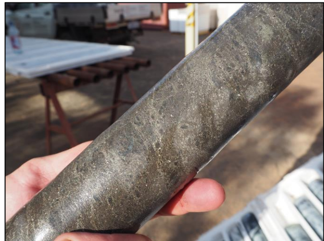
Photo 1 – 3: Massive pyrrhotite – pentlandite (nickel sulphide) – pyrite – chalcopyrite over 1.77m in drill-hole SNDD005 at Saint Patricks: 1.77m @ 6.72% Ni, 0.27% Cu and 0.13% Co from 227.31m down-hole.
