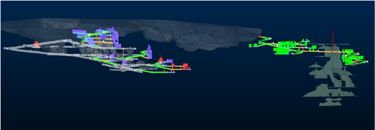
Figure 5 – Long section showing areas identified for mining. Dahmu Lode shown in purple, Hadfield Lode in green and Main Lode in green (north and south of historic stopping shown in grey)
