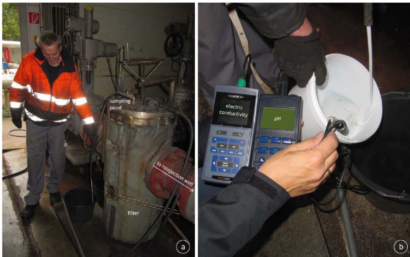
Figure 6: Confirmatory sampling of wells in Upper Rhine Valley by Vulcan team, and measurement of on-site brine parameters
