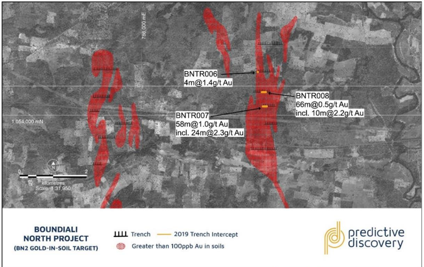
Figure 9 - Boundiali North targets BN2 and BN3 (at right and left respectively) with trench lines and significant results
