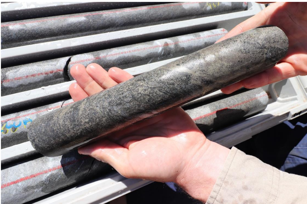
Figure 1: MDD334w1 core photo showing a section of massive and heavy matrix nickel sulphides
