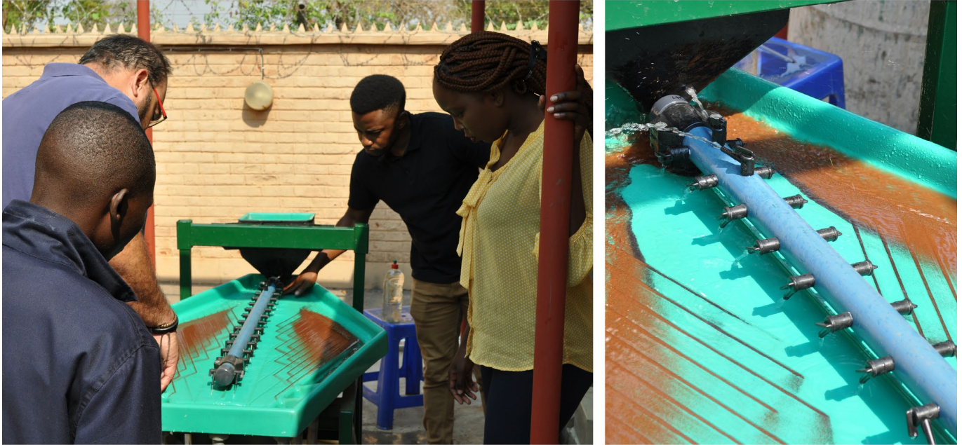
Figure 2 & 3: Wet tabling soil samples on-site in Malawi
