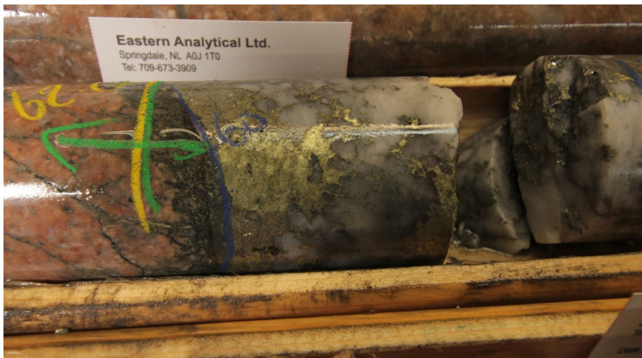
IMAGE 5: SULPHIDE MINERALISATION ENCOUNTERED IN HOLE CRD052 (showing chalcopyrite and pyrite within quartz veining)
