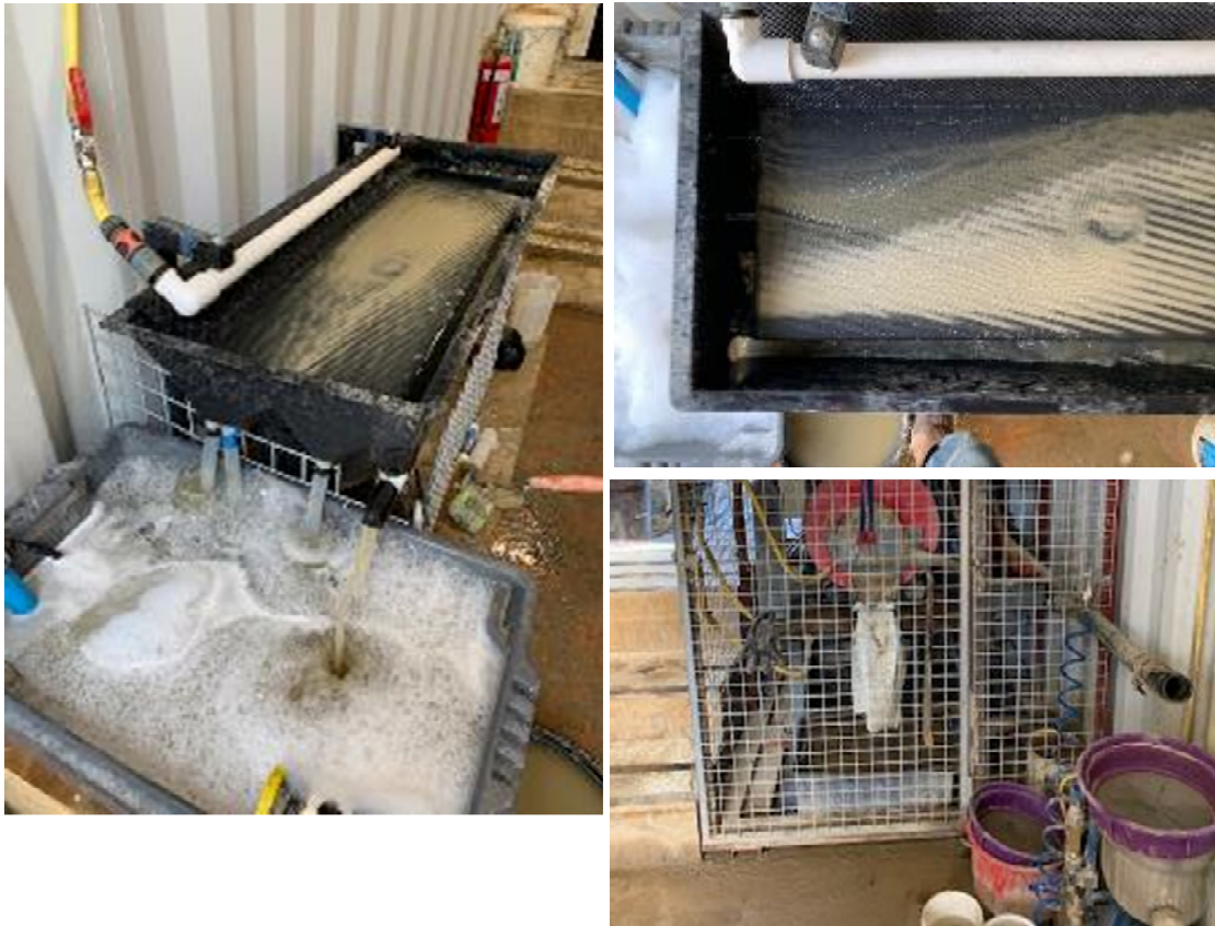
Figure 2: Photographs of the mill and shaker table
