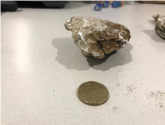
Picture 2: Taylor Lookout rock sample showing presence of Scheelite (most likely) under normal and UV light
