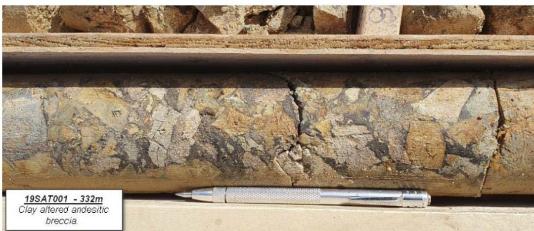
Figure 18 19SAT001 at 332m depth. Argillic alteration overprinting brecciated andesite.
