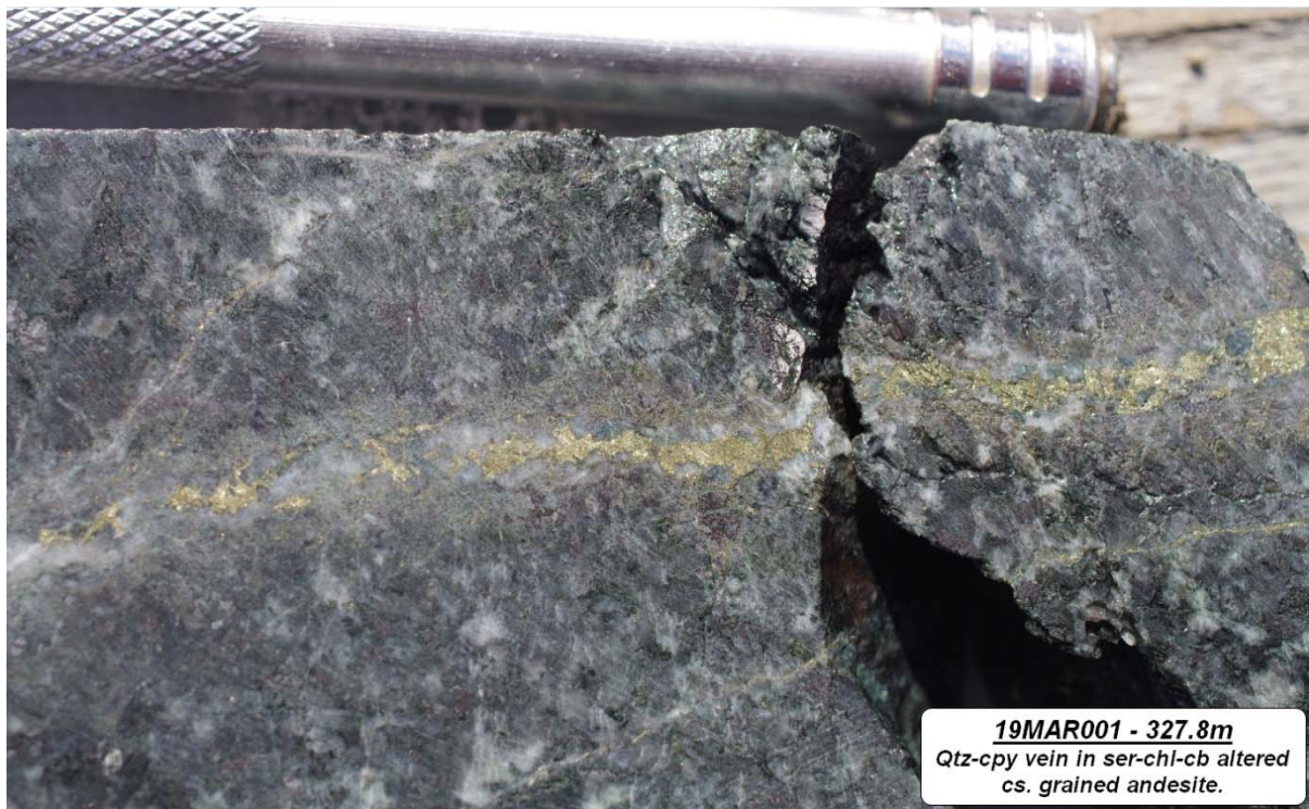
Figure 6 19MAR001 at 327.8m depth. Quartz-chalcopyrite vein in sericite-chlorite-carbonate altered diorite.
