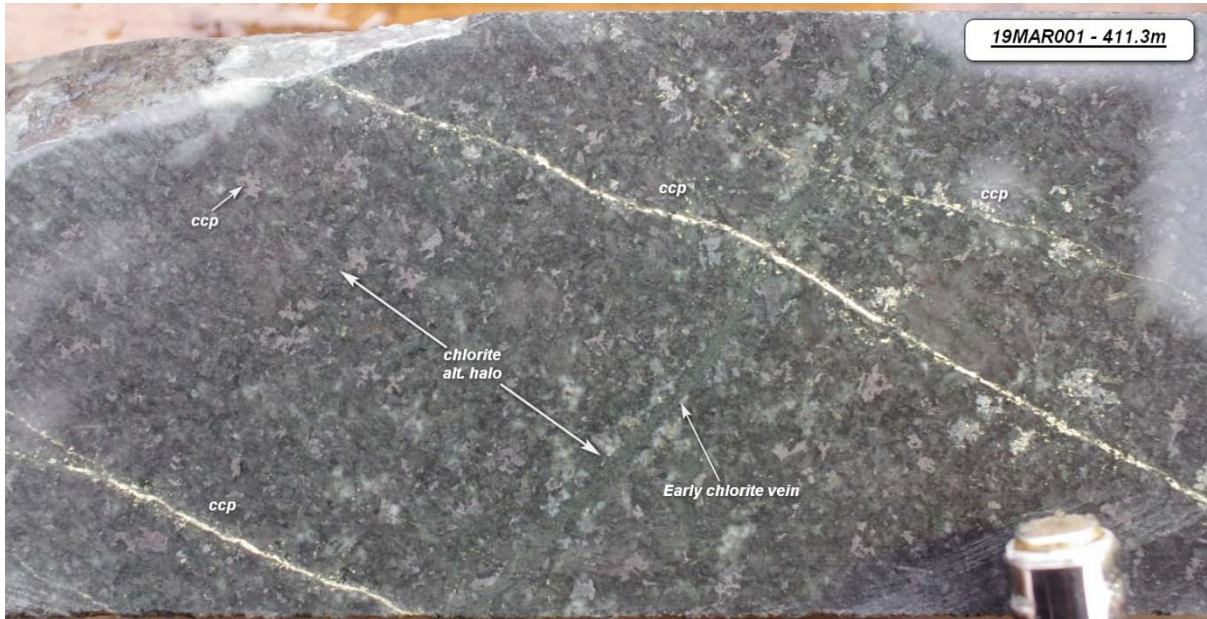
Figure 9 19MAR001 at 411.3m depth. Chalcopyrite veins in chlorite-magnetite altered diorite containing an earlier chlorite vein.
