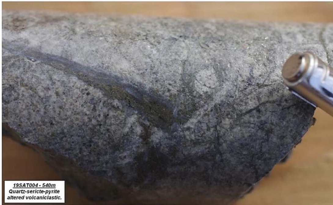
Figure 19 19SAT004 at 540m depth. Quartz-sericite-pyrite veining and alteration overprinting andesitic volcanic rocks.
