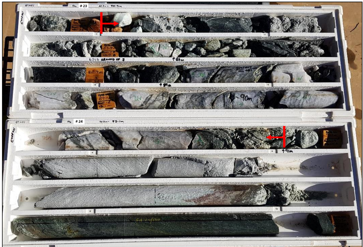
Figure 11. Quartz vein-shear hosted gold mineralisation within upper zone of EMD001 from 84.1m – 91.0m (6.9m @ 4.8g/t Au).
