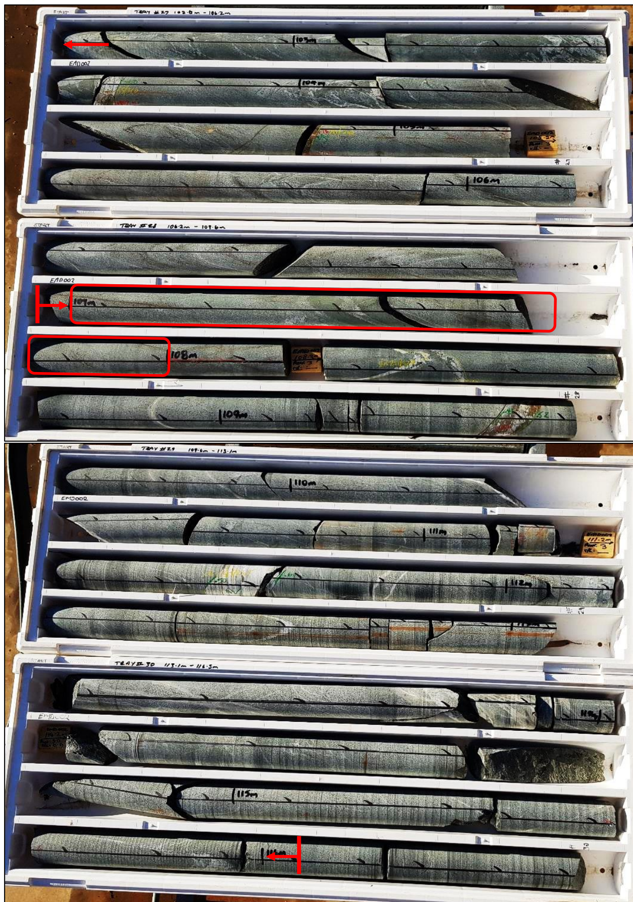
Figure 10: High-grade intersection in EMD002 which returned 16m @ 21.6g/t Au (102.0m – 118.0m). This includes “Bonanza Grade” intersection of 9m @ 35.9g/t Au from 107.0m – 116.0m (red arrows) which includes 1m @ 234.7g/t Au from 107.0 m – 108.0m (red outline).
