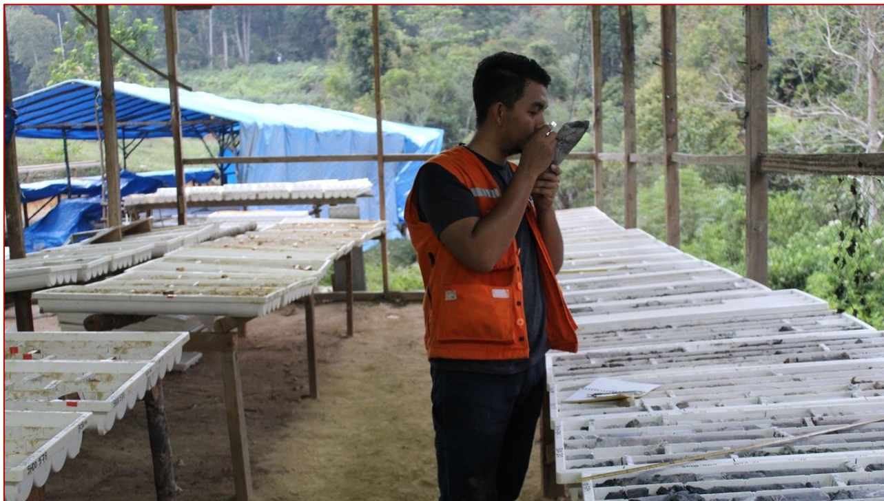
Photo 4 – Sihayo Gold Project core inspection and logging
