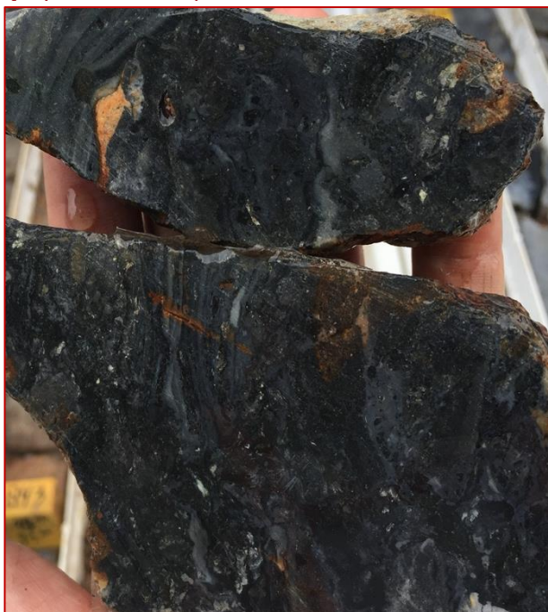
Photo 9 – SHDD564 at 102.5m down hole depth assaying 14.20 g/t Au (strongly sulphidic jasperoid breccia)
