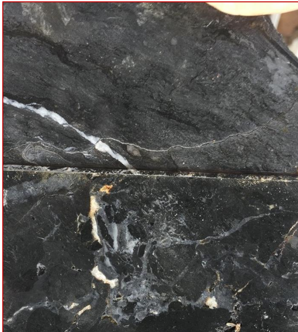
Photo 7 – SHDD564 at 96.5m down hole depth assaying 7.04 g/t Au (strongly sulphidic jasperoid breccia)
