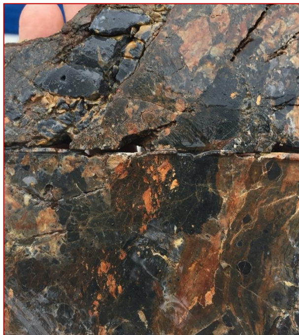
Photo 8 – SHDD564 at 100.5m down hole depth assaying 7.53 g/t Au (partly oxidised sulphidic jasperoid breccia)
