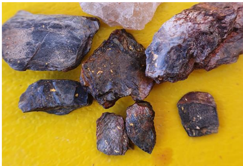
Visible gold flecks on RC drill chips from 19RRC035, 54-55m.
