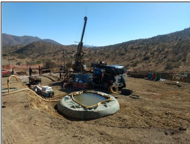
Photos 1 & 2: Diamond drill rig set up at Hole 1, Samuel Copper Project.
