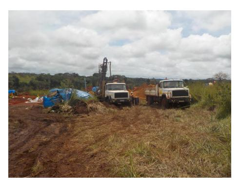
Photograph 1. Reverse Circulation drill rig setting up at drillhole PTRC002
