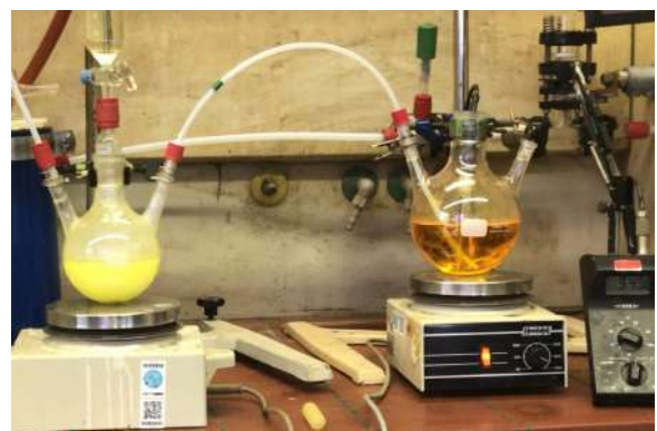
Figure 1: Oxidation to convert bromide ions using Cl gas Figure 2: Bromide ions converted into bromine
