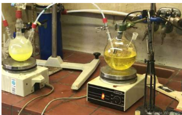
Figure 1: Oxidation to convert bromide ions using Cl gas Figure 2: Bromide ions converted into bromine
