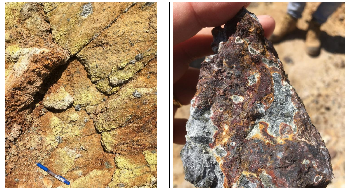
Figure 7 San Parami Mine; intense clay - sulphate altered granite with coarse grained pyrite (left) and partly oxidized silica-clay-pyrite rock (right).
