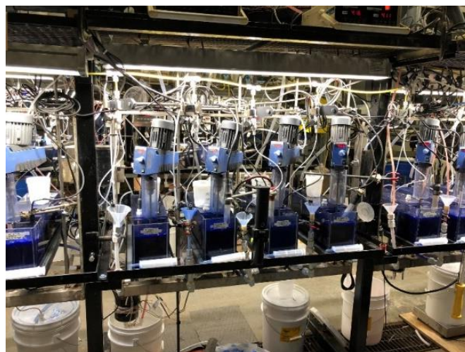
Figure 2 - Cobalt Recovery Circuit of the Neometals Pilot at SGS
