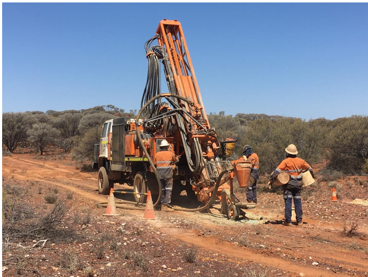
Figure 1 – Aircore drilling at Yuinmery Copper-Gold Project
