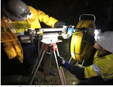
Figure 1: Full up-hole continuous gyro survey
