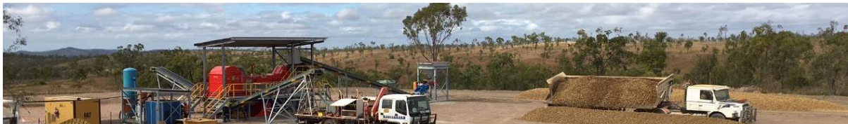
Figure 10: Tomra X-Ray Ore Sorter onsite at Far Fanning- ore sorting low grade stockpile material
