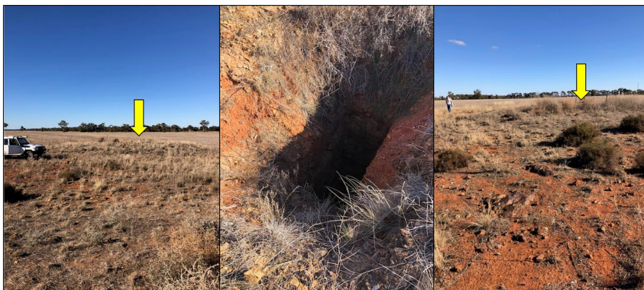
Figure 3: Tindall's Prospect: Yellow arrows define positions in photos of the two +50m deep historic shafts approximately 40m apart (E-W strike). Brecciated Ironstones sub-crops along this trend (similar to Collerina Deposit) - foreground of third photo.
