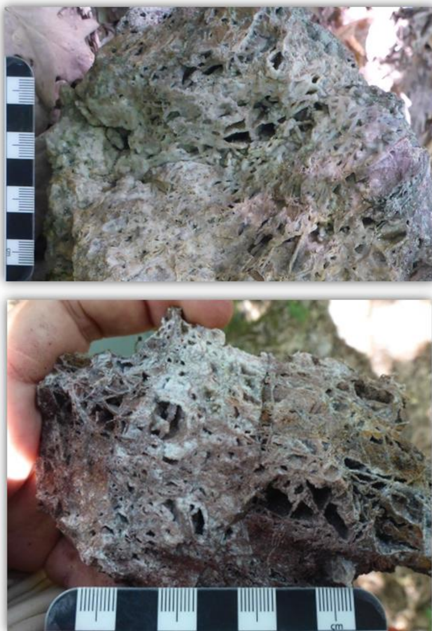
Figure 3: Rock samples from the Belopoltsi prospect displaying typical “lattice bladed” textures. This texture is typical of late replacement of carbonate by silica and indicative of a low temperature, low sulphidation epithermal depositional environment
