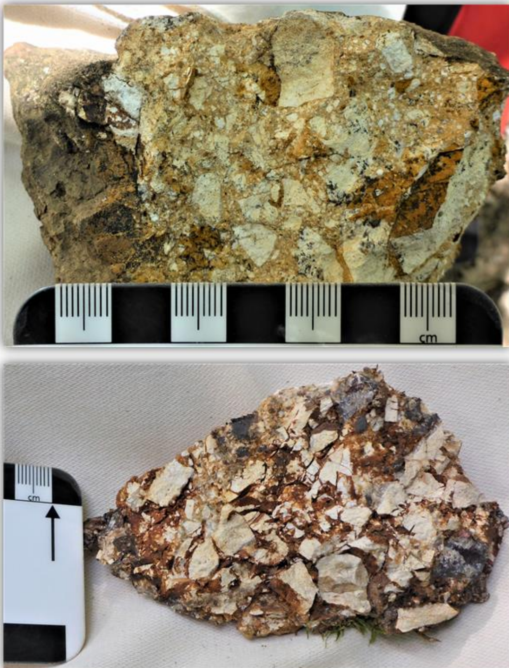
Figure 2: Hydrothermally and tectonically brecciated rhyolite from the Belopoltsi prospect
