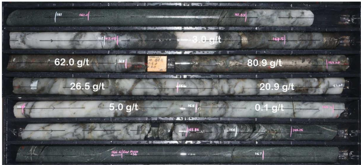
Figure 2: Drill core from Tribune infill diamond core hole DRDD257 high-grade mineralization associated with ~15% semi massive pyrrhotite, trace disseminated chalcopyrite and fine-grained visible gold. Interval assayed 9.6m @ 14.1 g/t gold from 107m.
