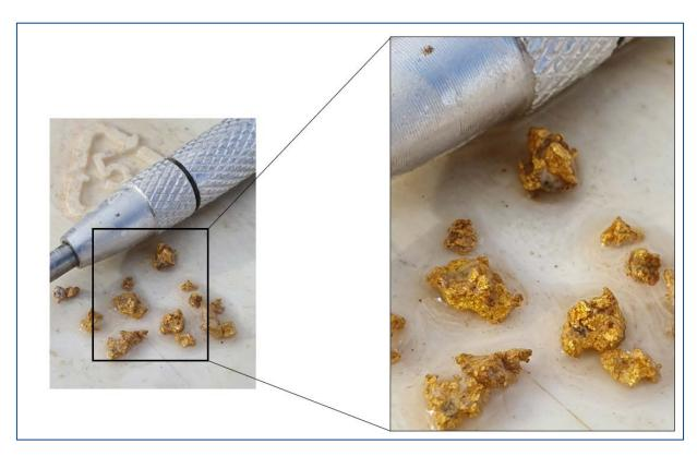
Figure 1 – Visible Gold in RC Chips from MLRC020 (from 3.0 - 3.5m interval)
