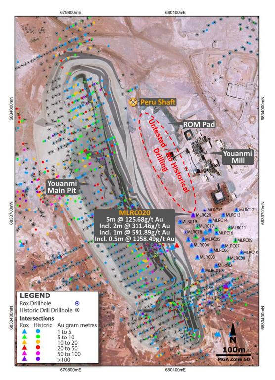
Figure 2 – Aerial photo with drill collars and intersections overlayed
