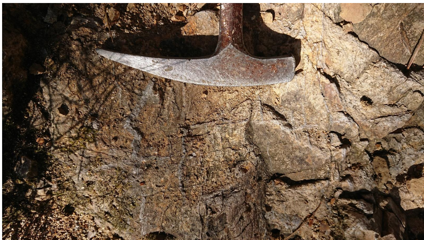
Figure 7 - Stockwork quartz veining within an altered diorite on the northern Sbor porphyry anomaly
