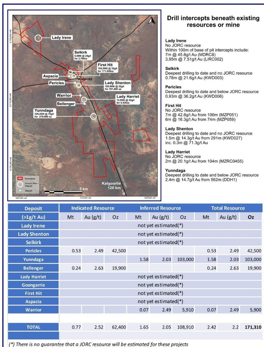
Figure 2: MGP historic underground and open cut mine production, current Mineral Resource Estimates (2016) and deepest significant drill intersections
