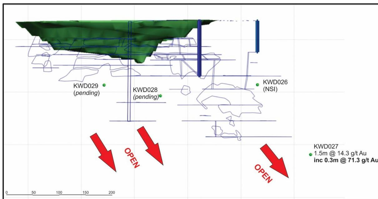
**Figure 1: Lady Shenton long section showing historic underground and open cut workings and KWR 2019 drill intersection points (N.B. only Lady Shenton lode shown, footwall and hanging wall lodes not shown)**
