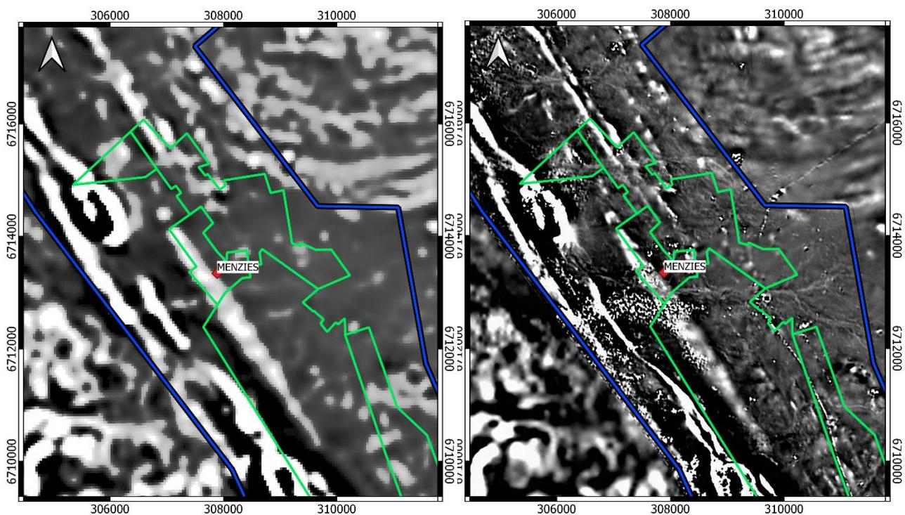
Figure 5: 100 metre lined spaced Government aeromagnetic survey on left and new 25 metre line spaced aeromagnetic survey on right (part of survey area only)
