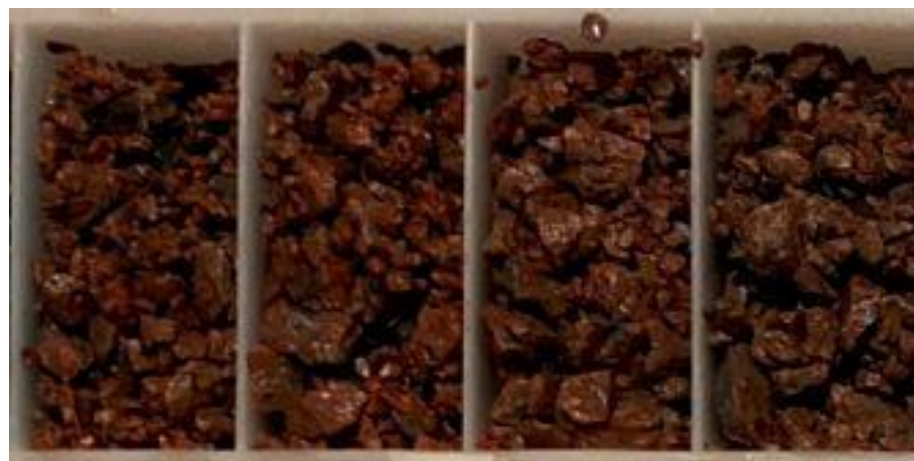
NMWBR18-010 204-208m. 4m @ 2.43g/t Au. Brick-red coloured hematitic alteration at contact of high-level porphyry intrusive and volcanic host rock
