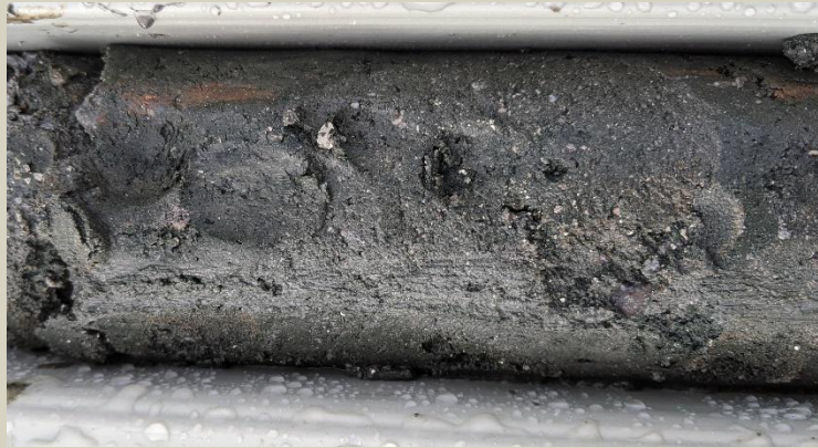
Green black clay with 2% disseminated pyrite and elevated Ni and Cr at 118m.
