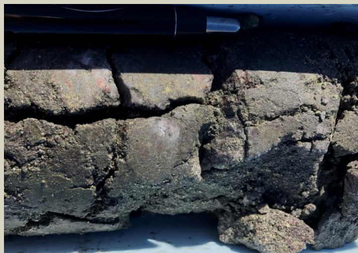
Semi-massive sulphide, pyrite+chalcopyrite in quartz+clay rock. 235.6m.
