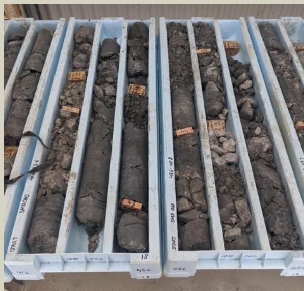
Broken zone of fracture-controlled sulphide and broken sandstone at 44m.
