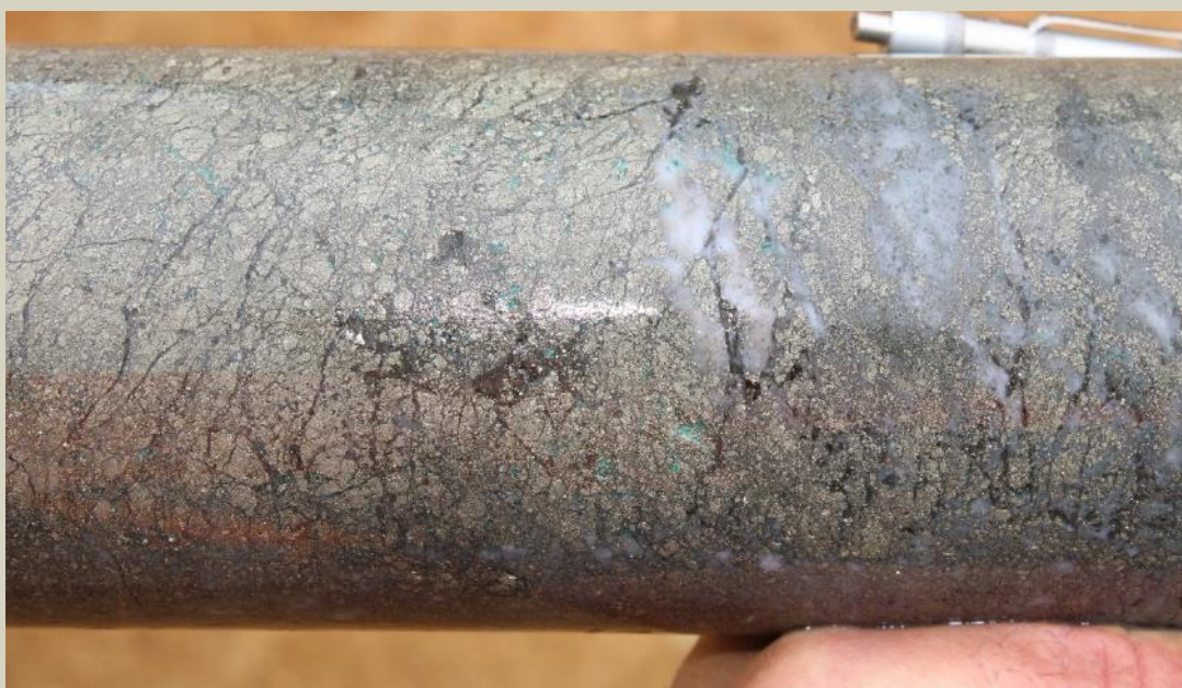
Massive to semi-massive pyrite+quartz with trace fuchsite and chromite grains at 68m.
