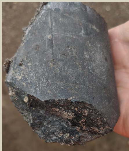
Sandstone with disseminated hematite/magnetite alteration and disseminated pyrite at 168m.
