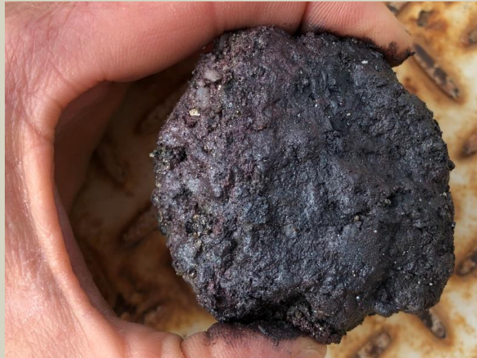
Hematite+specularite rock with disseminated pyrite and chalcopyrite. 199.8m.
