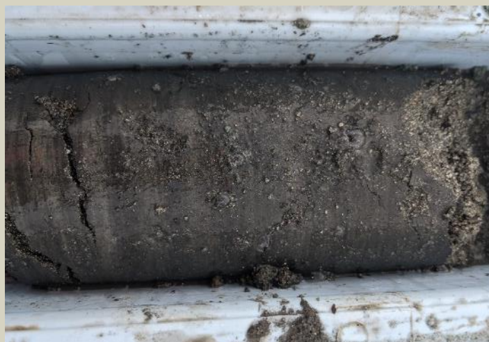
Friable massive pyrite zone at 65m.
