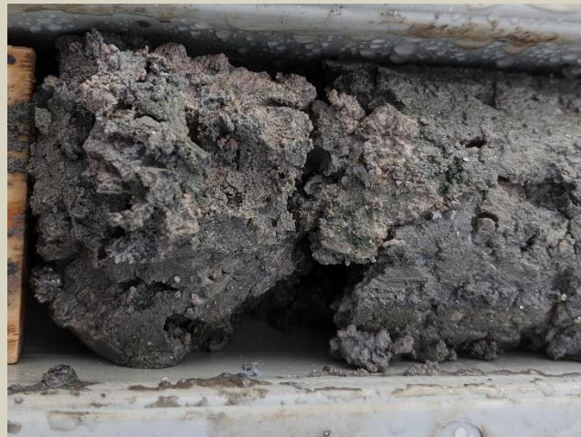
Strongly clay altered serpentinite at 118.5m.
