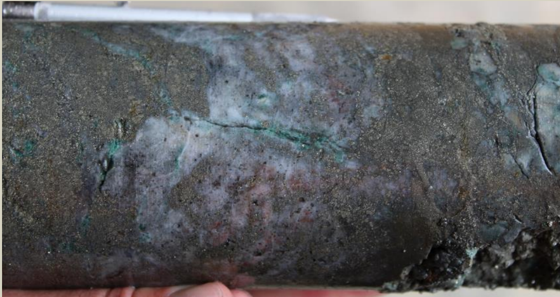
Semi-massive pyrite+quartz with weak hematite and trace fuchsite and chromite grains at 71.4m.
