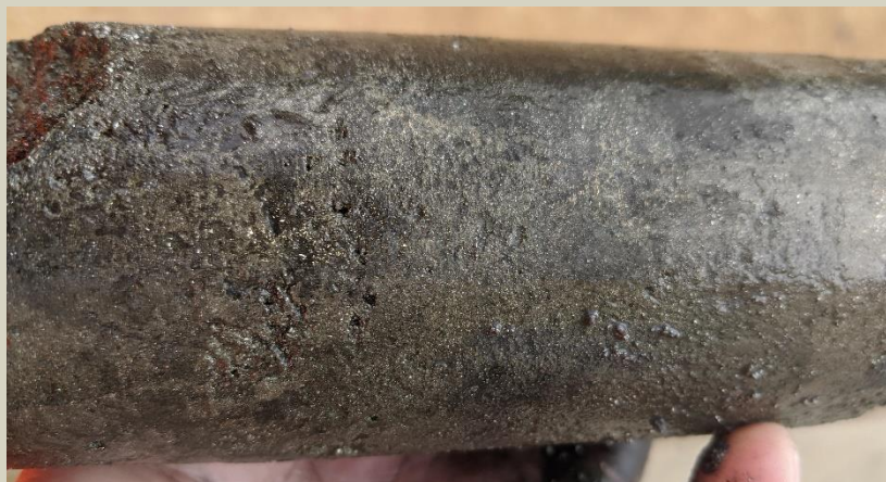
Massive pyrite with chalcopryite throughout at 81.8m.
