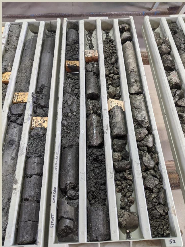
High grade mineralisation on the ultramafic contact from 129.9-135.15m.
