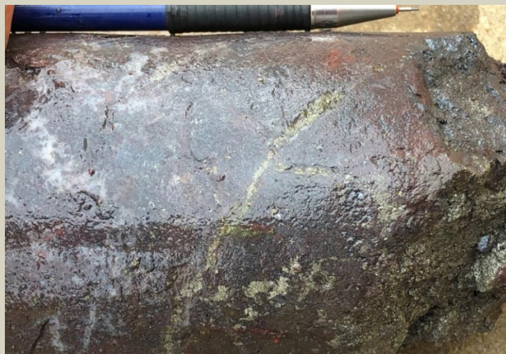
Chalcopyrite vein in hematite+specularite+quartz rock. 246.3m.
