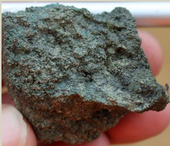
Chalcopyrite dominant part massive sulphide at 65.8m.
