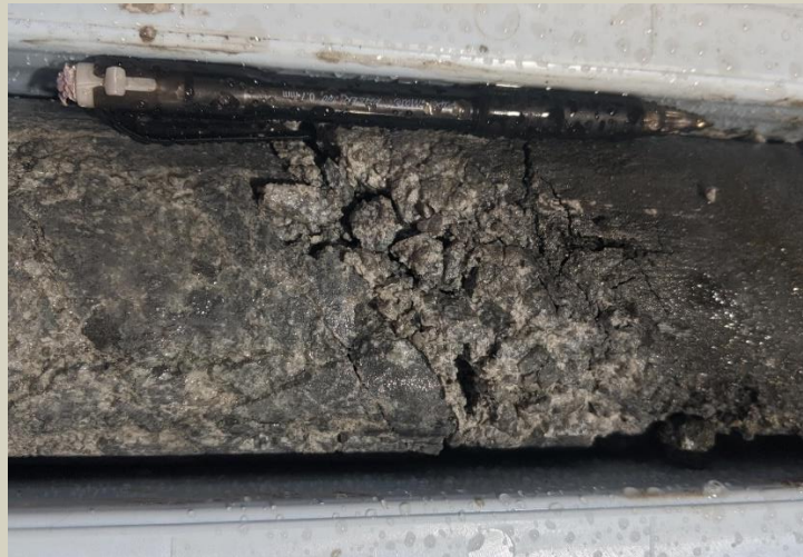
Pyrite and chalcocite on fracture surface at 61.9m.
