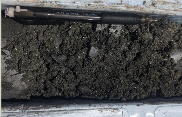
Massive pyrite/chalcocite vein at 66.2m.
