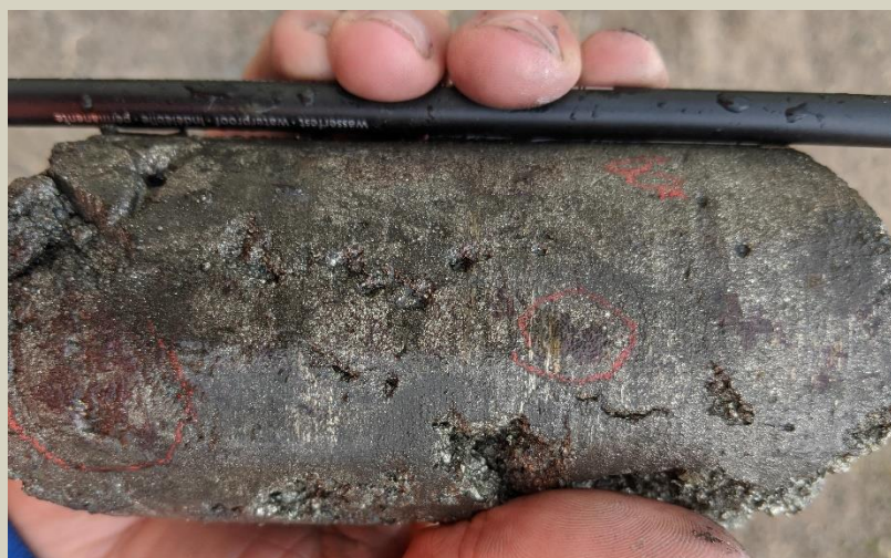
Massive sulphide with later bornite at 130.6m.
