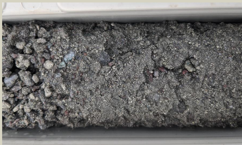
Friable massive pyrite mineralisation with hematite staining and silica alteration at 80.6m.
