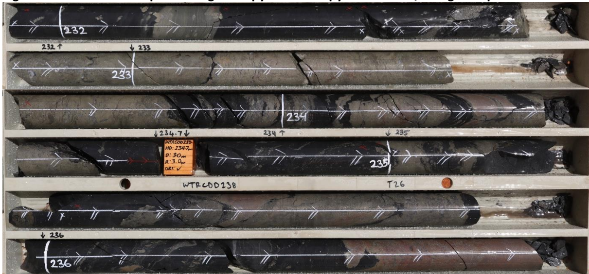
Figure 2 - WTRCDD238: Sphalerite-galena-pyrite-chalcopryite massive/stringer sulphides
