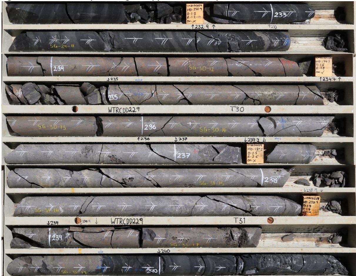
Figure 1 - WTRCDD229: Sphalerite-galena-pyrite massive sulphide
