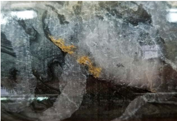
visible Gold in Drill core TDD015 at 90.4m
