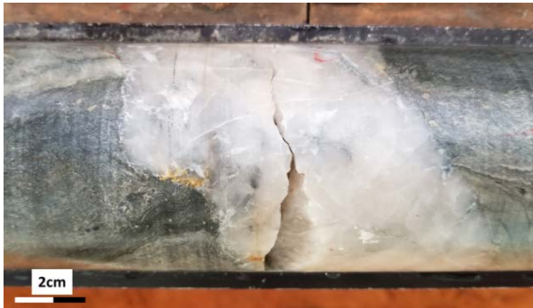
visible Gold in Drill core TDD013 at 129.8m
