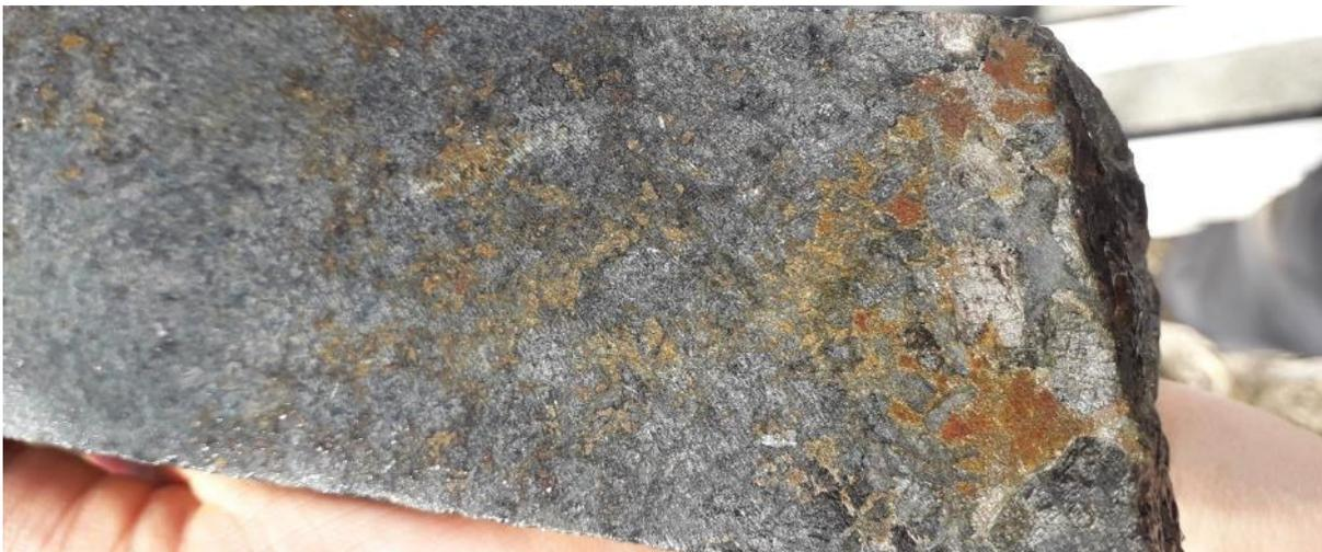
Figure 4. Net-textured sulfide from MRDD010 showing the 7cm section with high grade sulfide.
