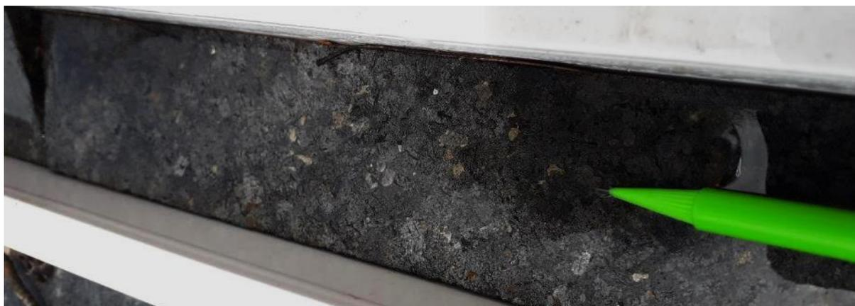
Figure 2. Coarse grained pyroxenite hosting interstitial sulfide from MRDD008 at 214m. Sulfides make up ~2-3 modal % of the rock. This intersection assayed at 0.11% Ni and 0.11% Cu.
