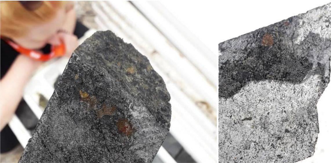
Figure 3. A. Large blebby sulfides from MRDD005 with some associated carbonate. B. Rounded globular sulfide from MRDD005 with inclusions and rims of carbonate. Dark surfaces are wet.
