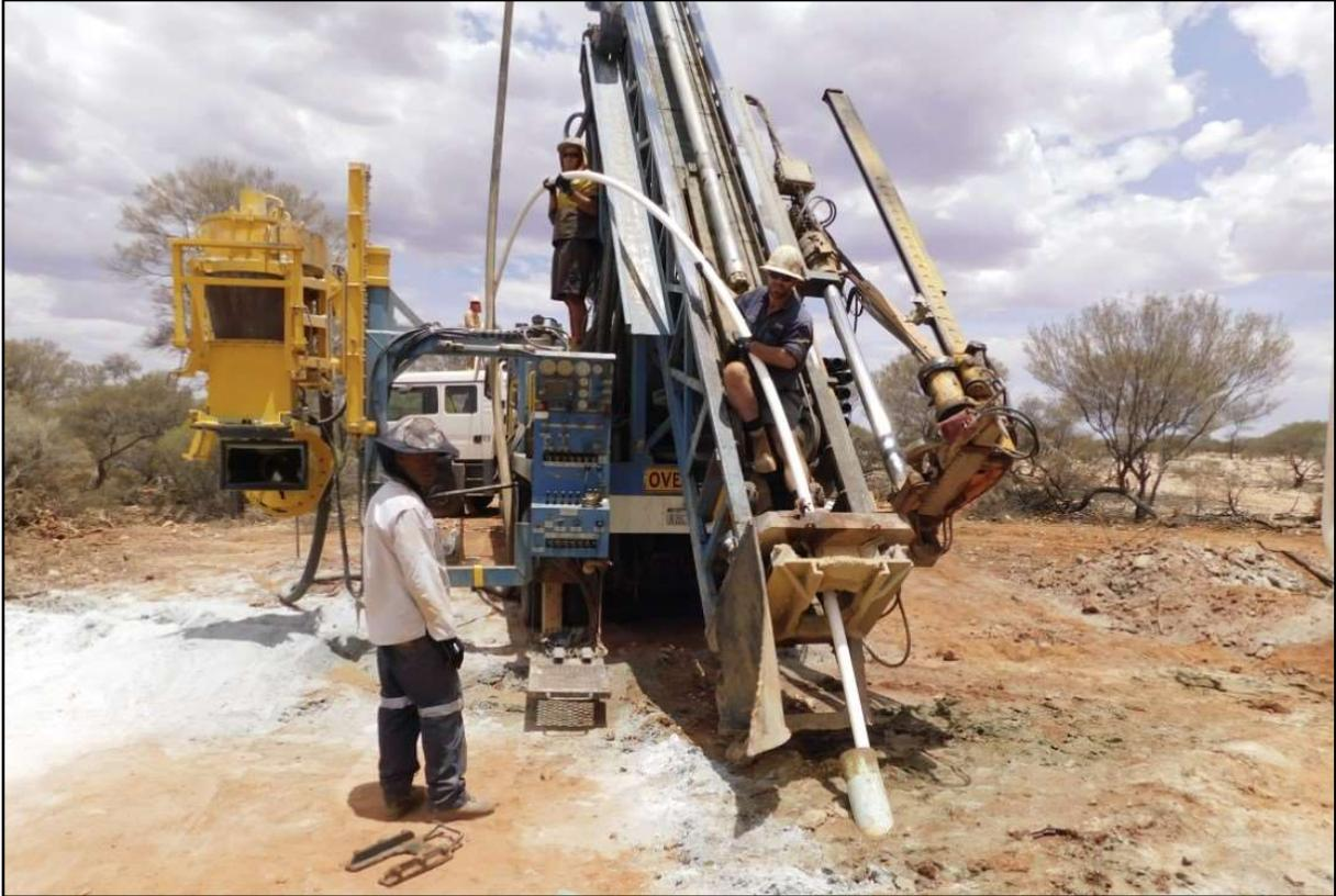
*Image 2 - Installing PVC casing in 19ESRC013 for downhole geophysical surveys*
