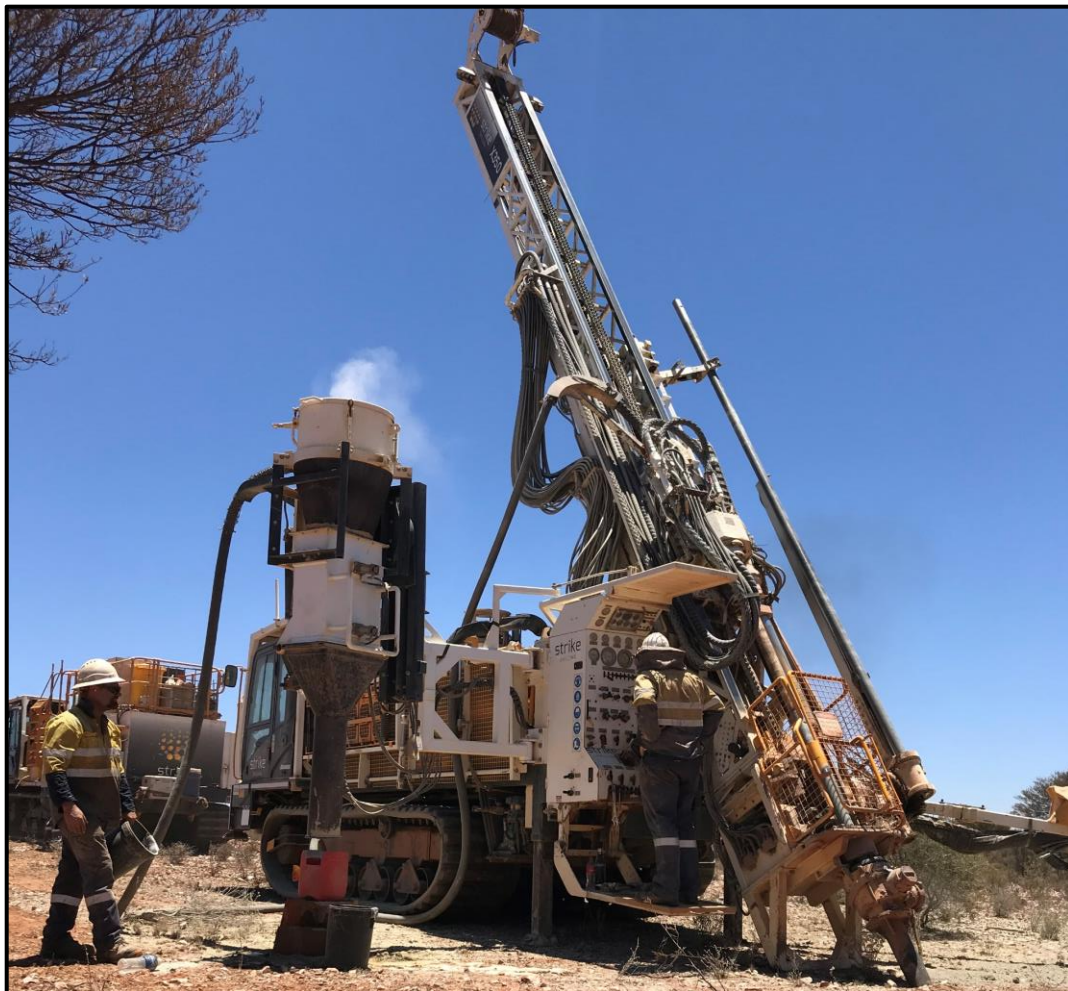
Figure 2: Aircore Drill Rig at the Four Mile Well Project.
