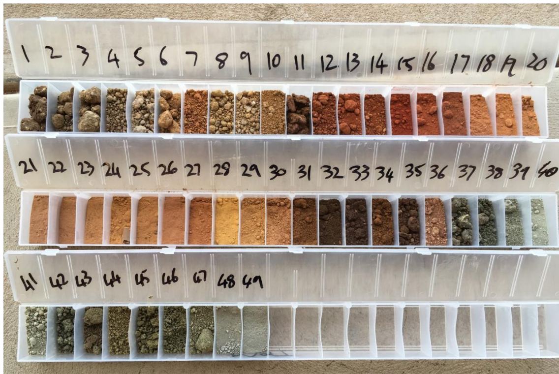
Figure 3: Drillholes MA07 chip tray samples – representative of intersected lateritic material
