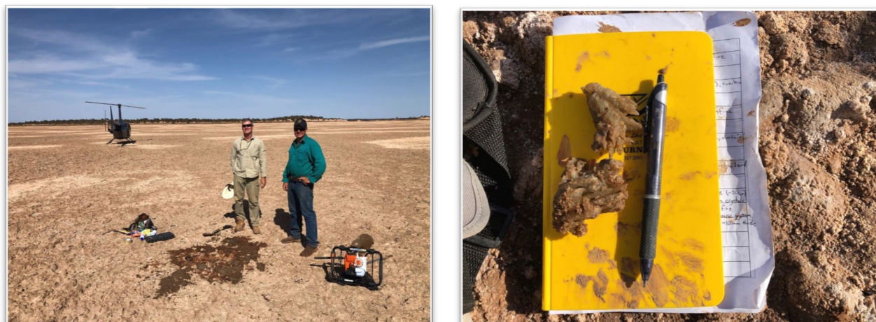
Figure 1: Showing sampling activities over Lake Throssell (LHS) and an example of gypsum crystals identified in the field (RHS)
