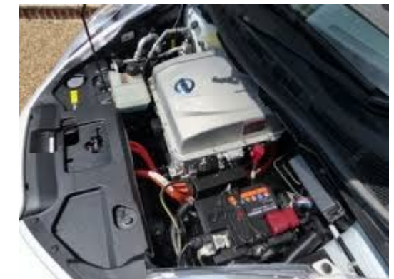
The engine bay of a Nissan Leaf – note the lead-acid battery centre bottom (image: autonews.uk.com)
